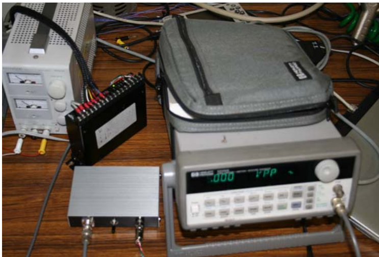
Figure 1: Electronics used: The stepper motor driver (black box) and function generator (device with digital display) are connected by the switching box (lower left corner).
