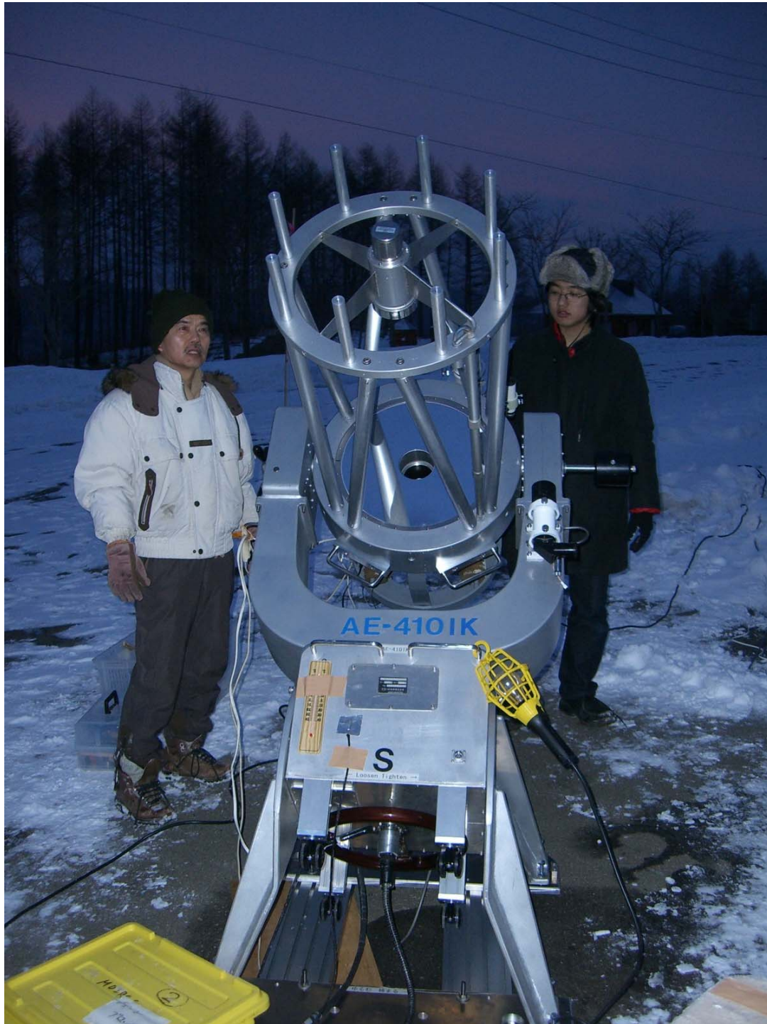
AIR-T-40 40 cm Antarctic Infra-Red Telescope
