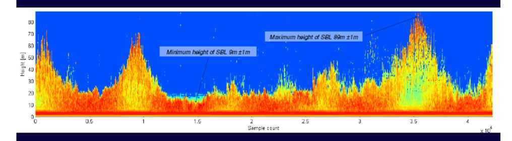
Six days of processed data from acoustic radar (Snodar)
