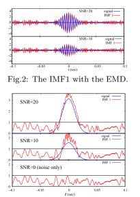
Fig.3: The instantaneous amplitude of IMF1 with the EMD.
