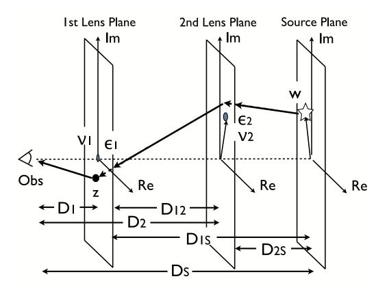
Figure 1: Notation: The source and image positions on complex planes are denoted by w and z, respectively. Locations of N masses are denoted by  $\epsilon_i$  for  $i = 1, \dots, N$ . Here, we assume the thin lens approximation for each deflector. The several distances among the observer, source and each lens object are also defined.
