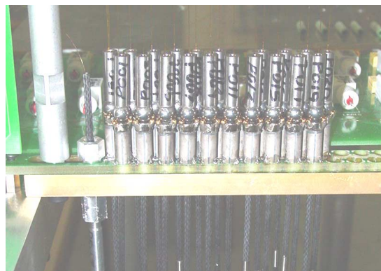
Fig. 13: Left: the half-filled prototype module. The LEDs for back-illuminating the fiber are to the right. Right: a close-up of the half-filled module, showing the required packing density of the spines in Echidna.
