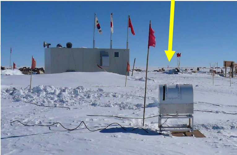
Radiometer Transmittance of atmosphere
