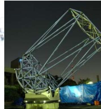
2m Infrared Telescope
