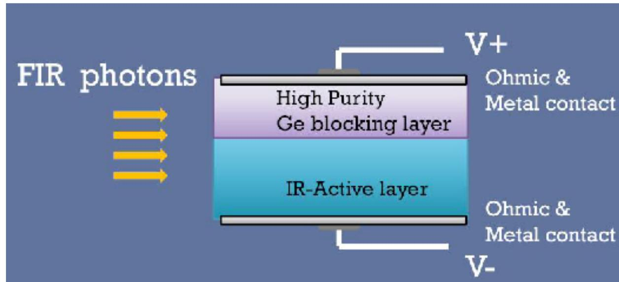
develop ohmic contact by AuGe deposition
