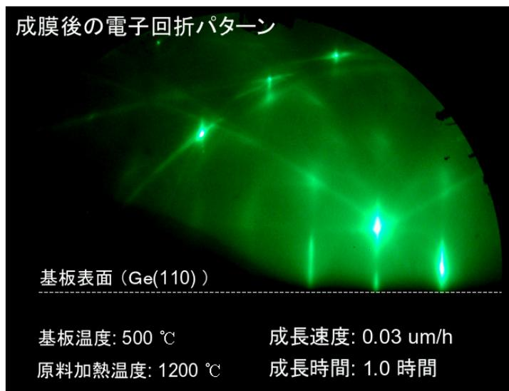
Reflection High Energy Electron Diffraction (RHEED)
