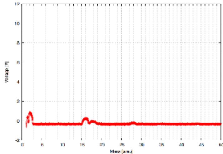
Quadrupole Mass Spectrometer (QMASS) analysis results
