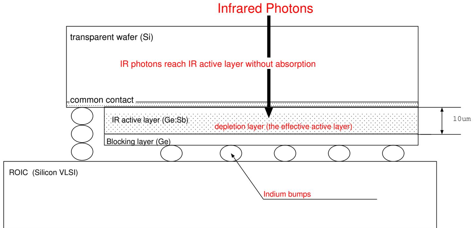
IR photons goes to directly to the active layer (no phonon absorption!)
