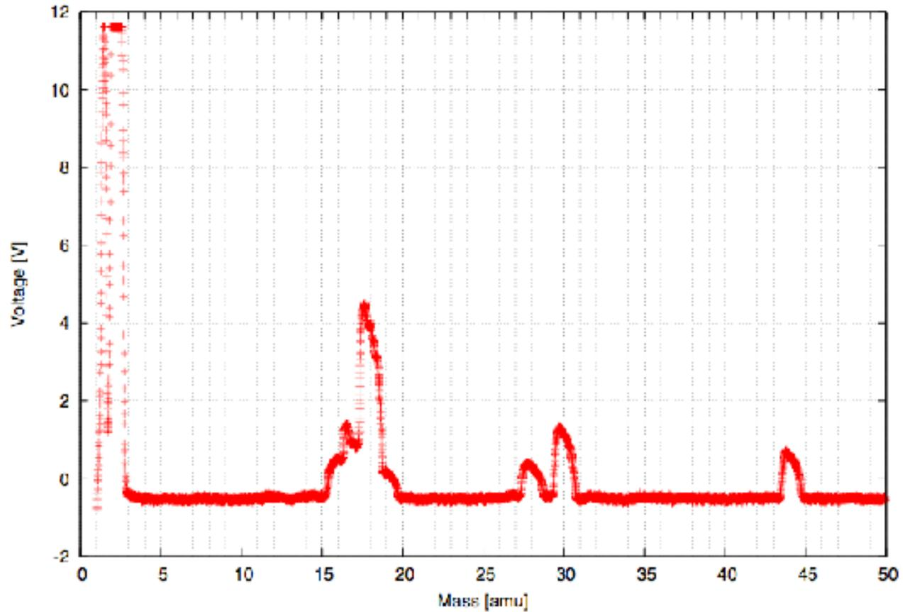
Quadrupole Mass Spectrometer (QMASS) analysis results
