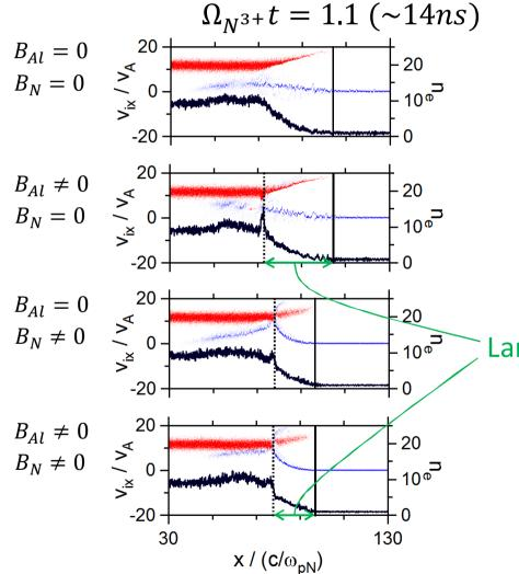
Finite  $B_{Al} \neq 0$  is necessary to form  $n_e$  jump for  $B_N = 0$
